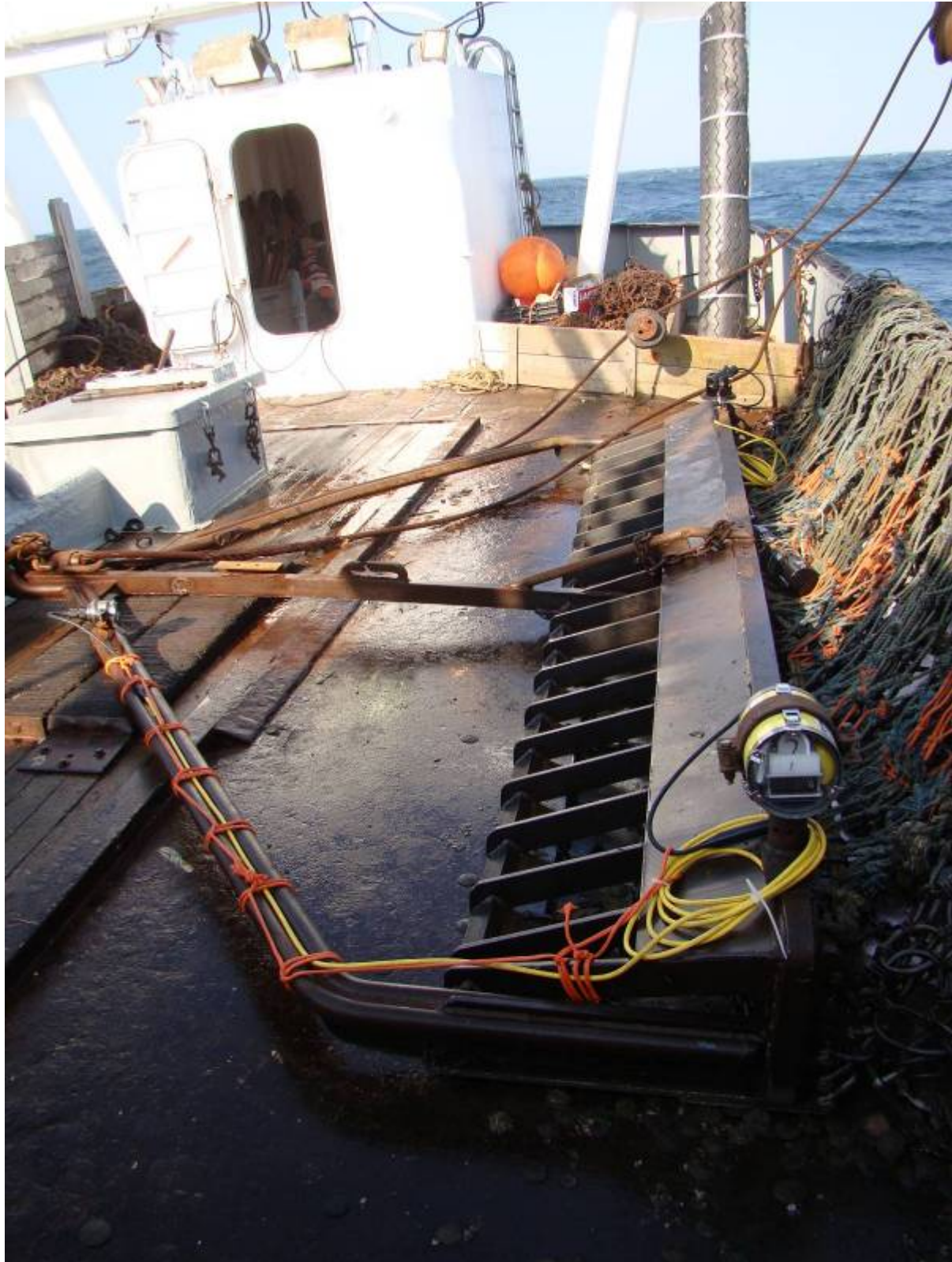
Figure 2: Low-profile dredge showing the placement of cameras during CFRF Challenge Grant video trials.
