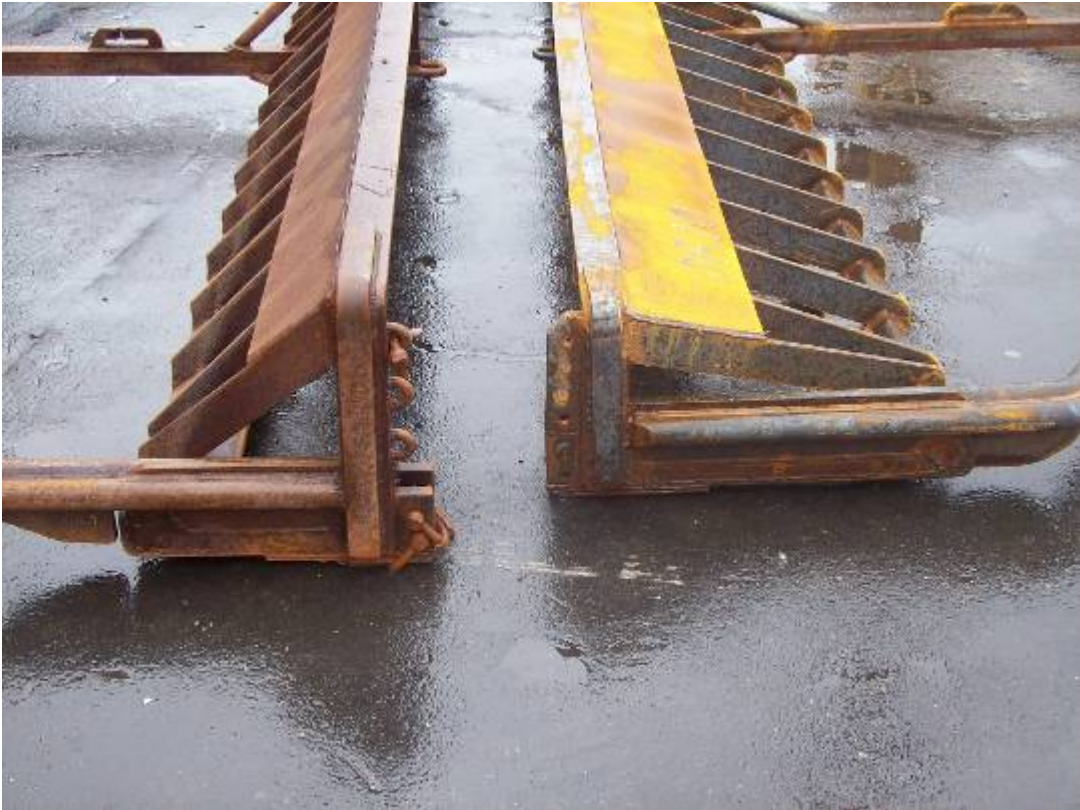
Figure 1: Comparison of the low profile dredge to the Cfarm Turtle Excluder Dredge.
