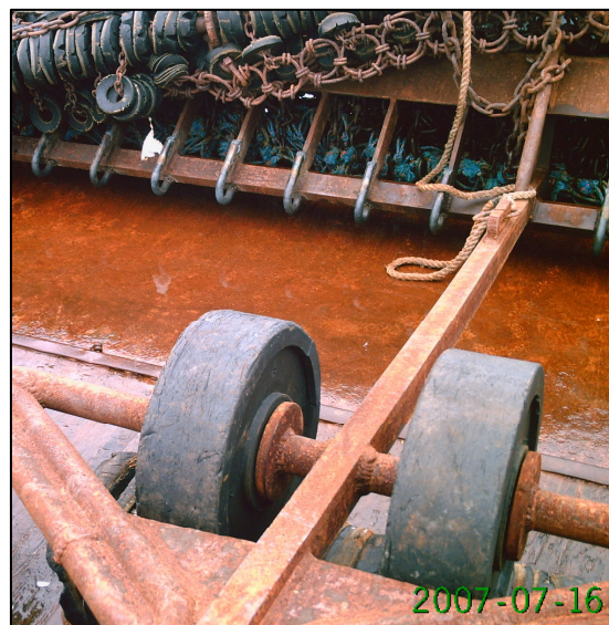
Figure 1. Experimental dredge design 3 with turtle guards on the cutting bar and a doubled outer bale.
