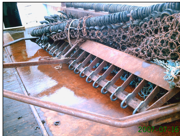
Figure 1. Experimental dredge design 3 with turtle guards on the cutting bar and a doubled outer bale.
