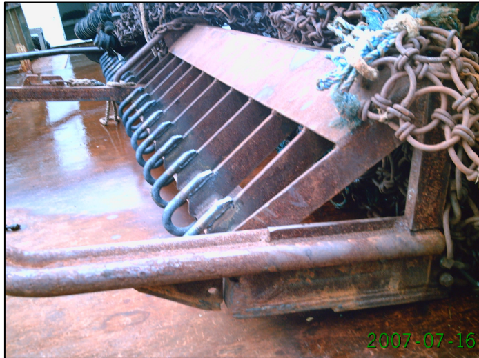
Figure 3. Side view of shoe used; the shoe was 1/2" x 3" spring steel cut 17 1/2" long and attached to 1 1/2" x 3 1/2" x 15" long bar stock
