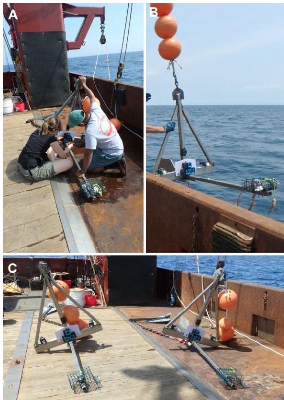
Figure 7. BUV frame. (A) Setting up for a drop. (B) BUV frame going over the side with dangling squid bait. (C) Both BUV frames set up with Danforth anchors.
