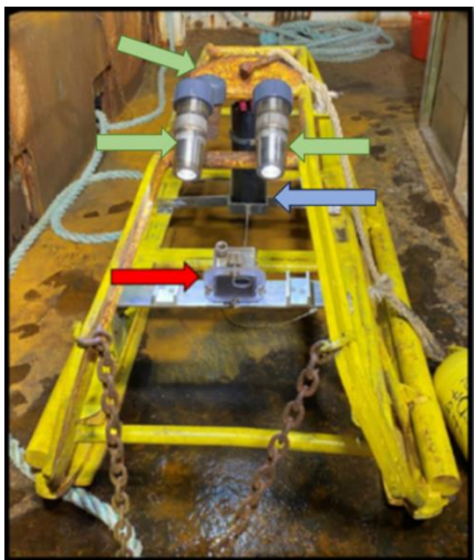
Figure 7. CFF benthic sled built in 2014. Red arrows indicate the location of the forward-facing camera, blue arrow indicates the location of the bottom-facing camera, and green arrows indicate the location of lights.
