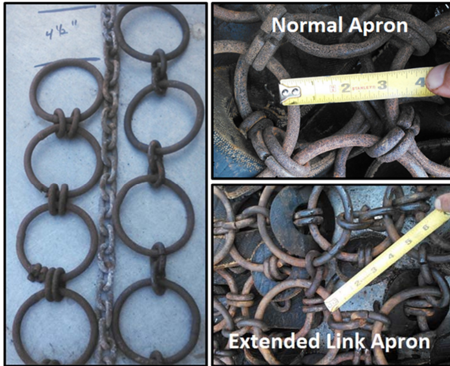
Figure 1: (Left) A side-by-side comparison of a row of rings from a normal apron and the extended link apron. (Right) The inter-ring spacing in a normal apron and a two-way extended link apron.
