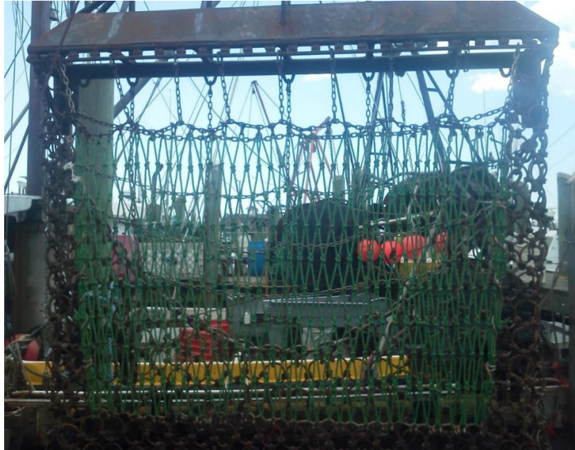
Figure 1. Location and configuration of the row of 12 inch windows behind the dredge frame.
