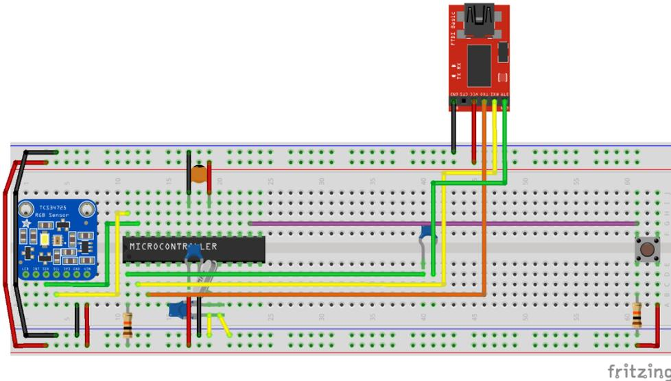
**Figure 10.** Breadboard diagram of the colorimeter, the microcontroller is an ATmega328 which interprets the sensor values and outputs them via an FTDI adapter.
