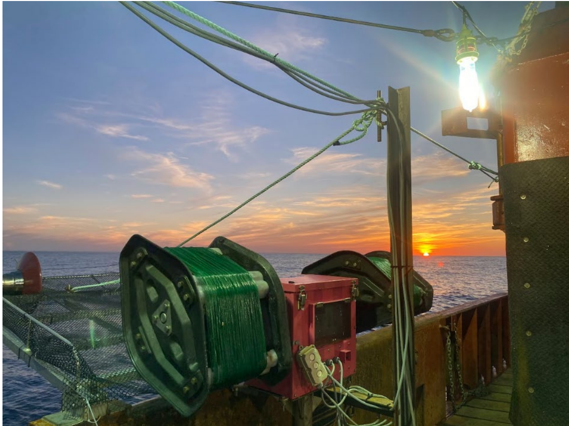
A double-drum automatic jigging machine with overhead metal halide lighting begins fishing at sunset.
