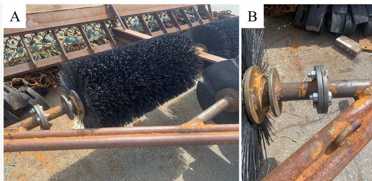
Figure 6: The street sweeper sweep mounted to a TDD (A) and a close up view of the mounting mechanism (B).
