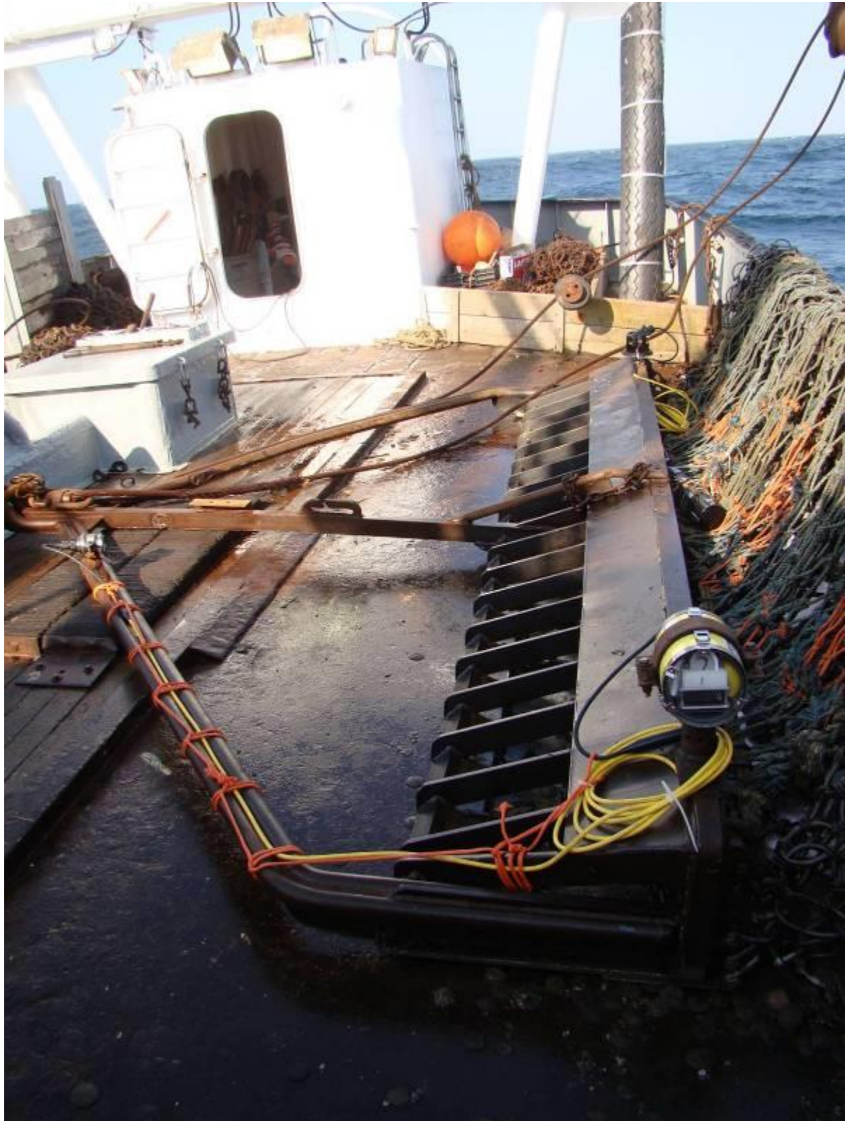
Appendix A2: Low-profile dredge showing the placement of cameras during CFRF Challenge Grant video trials.
