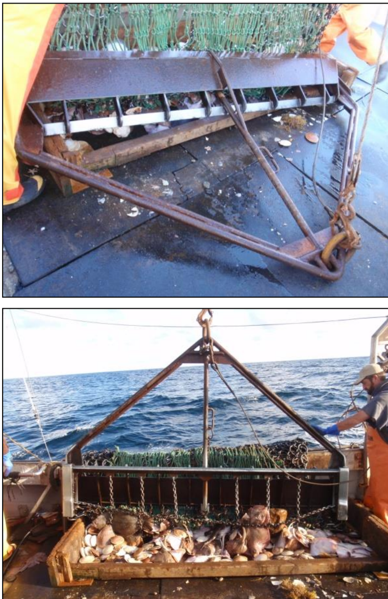
Figure 1: Upper and under side of the Coonamessett Farm Low Profile 9-foot dredge.
