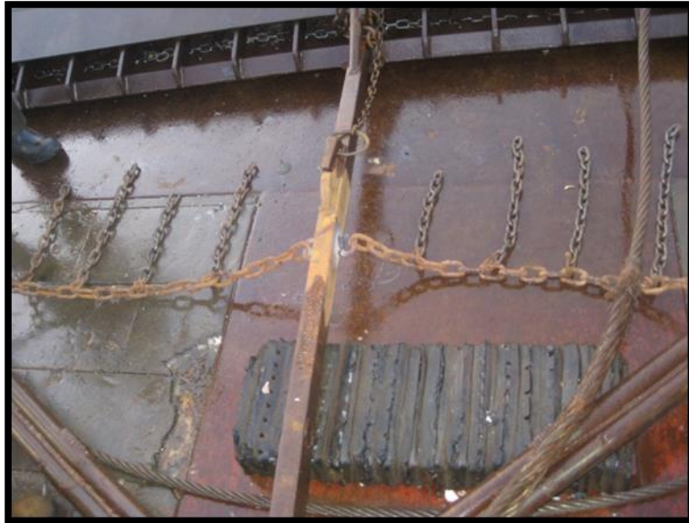
Figure 5: The Forward Tickler Chain design that was tested aboard the F/V Weatherly. (Note the wide depressor plate at the top of the photo.)
