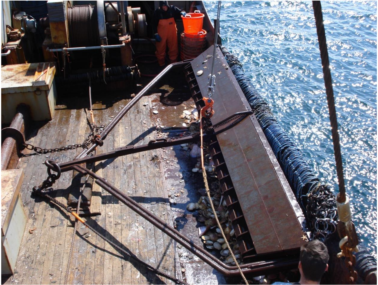
Appendix A3: Low-profile dredge showing the wider (20-inch) depressor plate used in the LA research trips.
