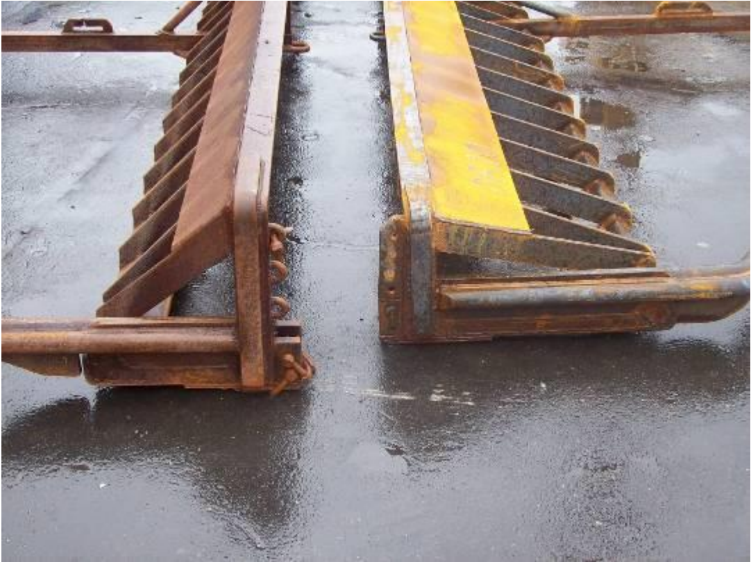
Appendix A1: Comparison of the 15-foot low profile dredge CFLP(Left) to the Cfarm Turtle Excluder Dredge (Right) (8 inch wide depressor plates).
