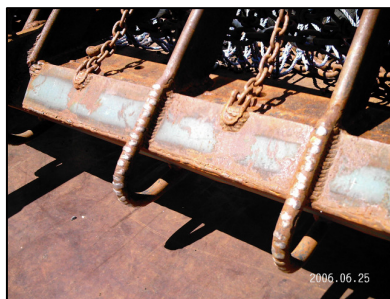
Figure 4. Photograph of the cutting bar used on experimental dredge frame design 1 (left) and a view of cutting bar used on a New Bedford dredge (right)
