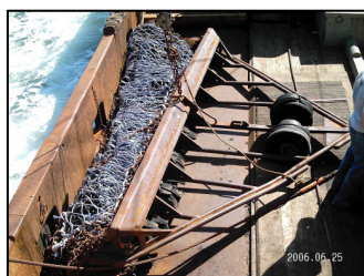
Figure 20. Photograph F/V Celtic's New Bedford dredge used as control (left) and experimental dredge frame design 1 (right)
