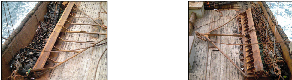
Figure 23. Photograph F/V Westport's New Bedford dredge used as control (left) and experimental dredge frame design 2 (right)
