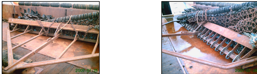
Figure 25. Photograph F/V Friendship's New Bedford dredge used as control (left) and experimental dredge frame design 3 (right)
