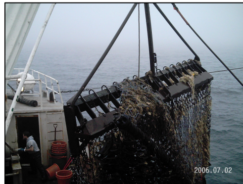
Figure 26. Photograph showing the twine top being hung up on the turtle guards
