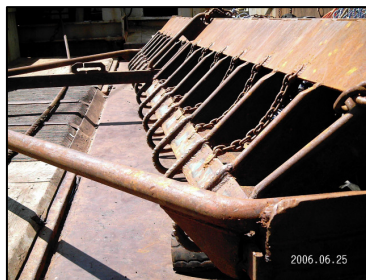
Figure 3. Photograph showing the position of the cutting bar relative to the pressure plate on experimental dredge frame design 1 (left) and the New Bedford dredge (right)
