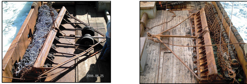
Figure 22. Photograph F/V Celtic's New Bedford dredge used as control (left) and experimental dredge frame design 2 (right)
