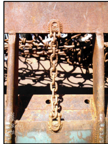
Figure 9. Photograph of the frame chains on experimental dredge design 1
