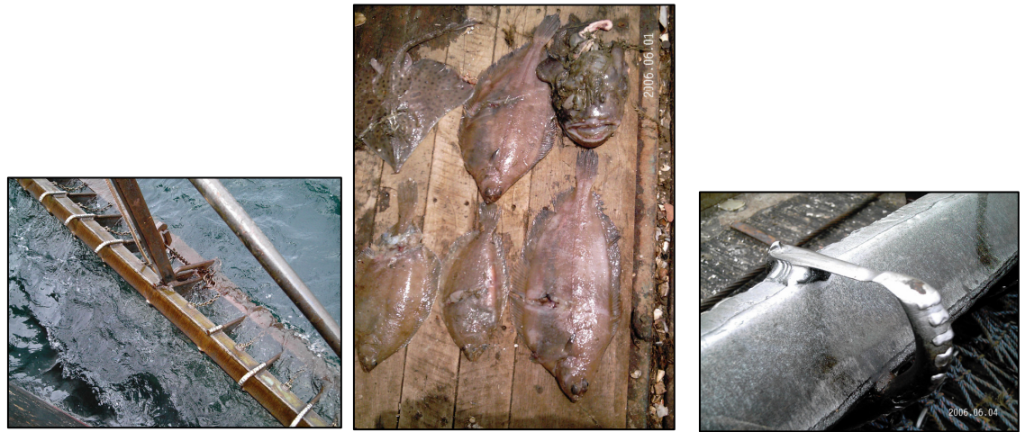
Figure 27. Photograph showing the wearing down of rebar loops used for the turtle guards (right and left) and fish cut by the turtle guards (center)
