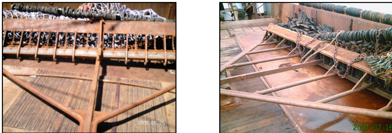
Figure 6. Photograph of the bale used on experimental dredge frame design 1 (left) and a the bale bars used on a New Bedford dredge (right)
