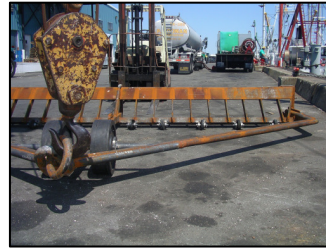
Figure 24. Photograph F/V Friendship's New Bedford dredge used as control (left) and experimental dredge frame design 3a (right)
