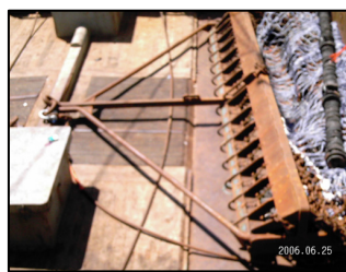
Figure 20. Photograph F/V Celtic's New Bedford dredge used as control (left) and experimental dredge frame design 1 (right)
