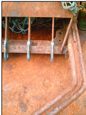
Figure 16. Photograph of bale extension used on experimental dredge design 3
