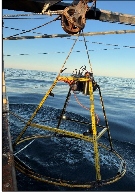
Figure 2. Drop camera array used to survey the Davis Bank East research area in the Great South Channel Habitat Management Area.
