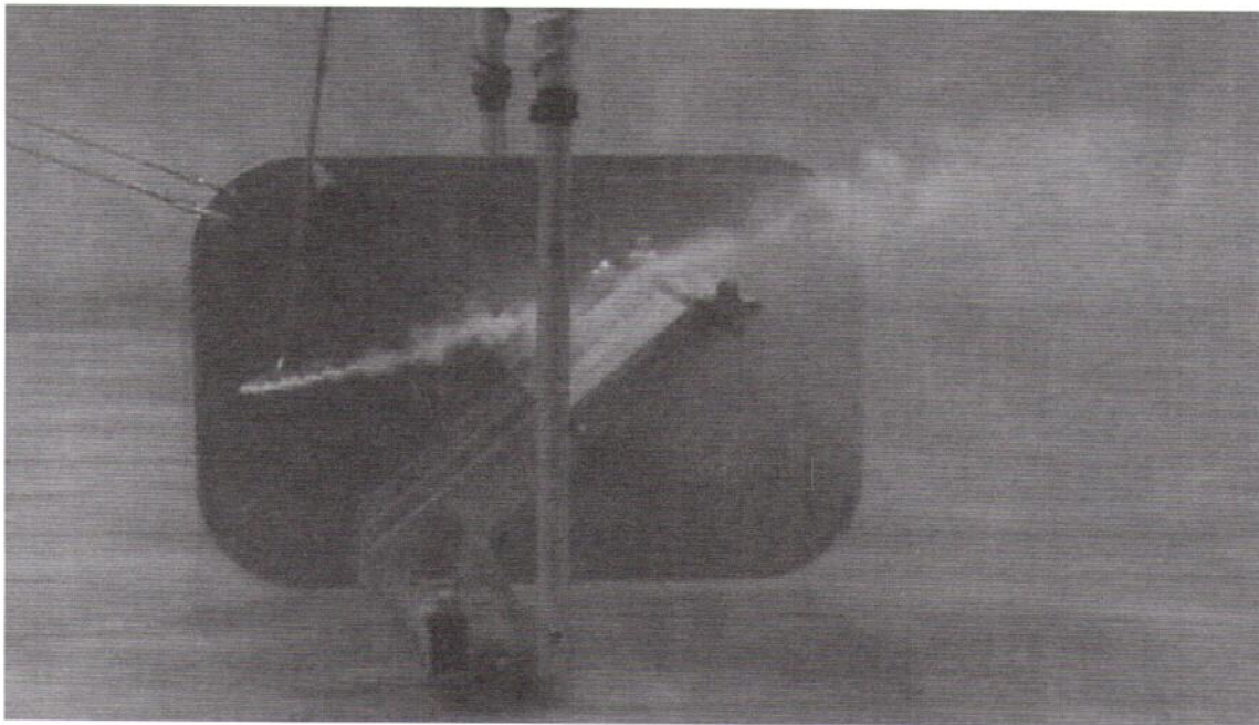
FIGURE 4. Panel (A) shows the experimental dredge frame design used in the flume tank tests. The major components are labeled for reference. Panel (B) shows a dye injection test that illustrates the hydrodynamic flow around the depressor plate; the water flow hits the plate and is ramped up and over the dredge. [Figure available in color online.]
