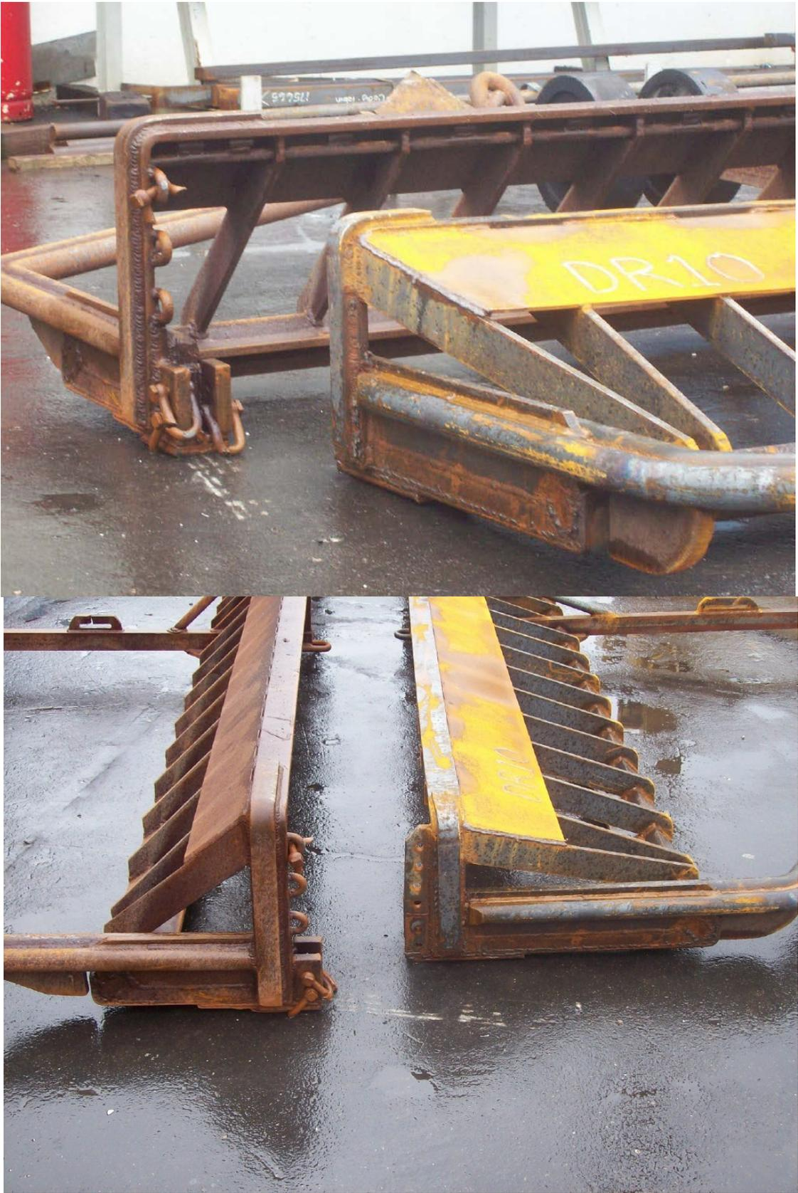
**Figure 2:** Basic Low profile design with standard 10-inch depressor plate.
