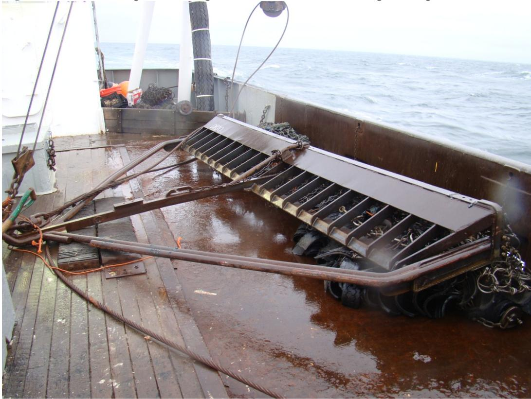
**Figure 3:** Wide depressor plate (20-inch) design.
