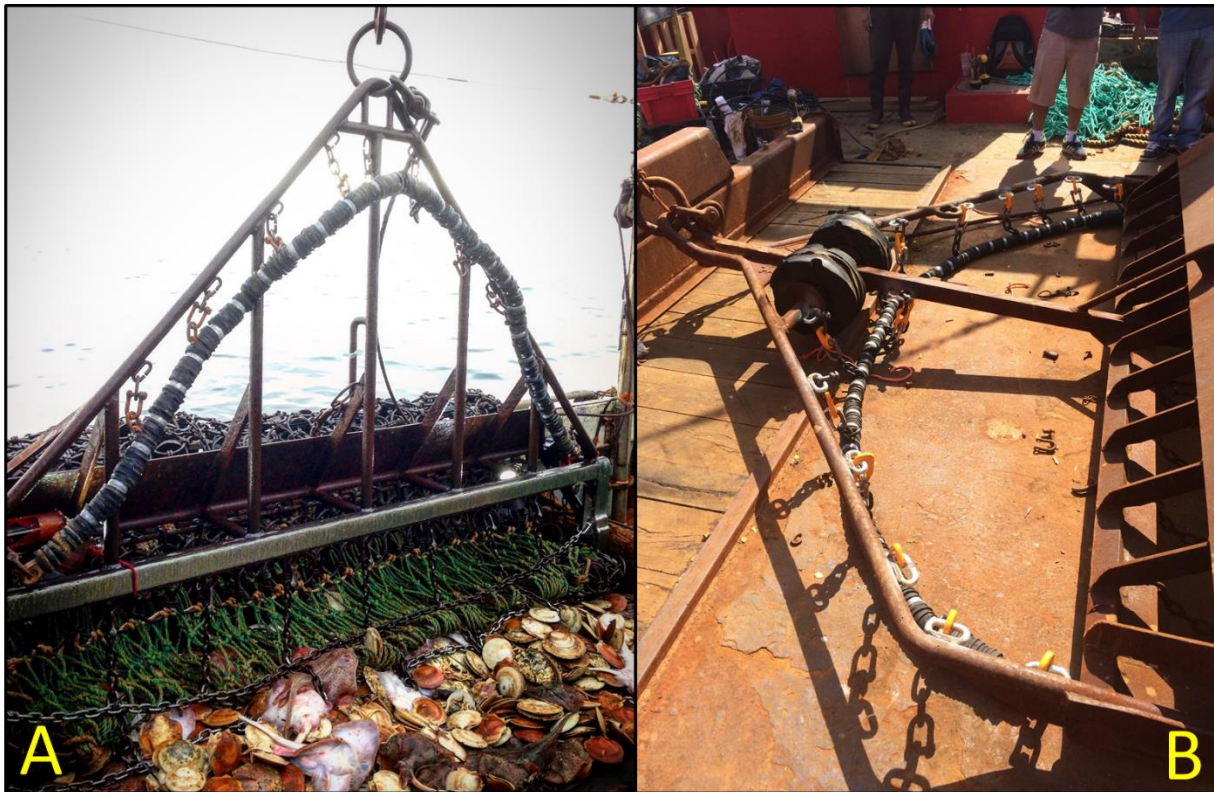
Figure 1. A 9' sea scallop dredge equipped with a flounder cookies sweep (FCS) attached along the outer bale bars aboard F/V Mister G (A) and an 11' sea scallop dredge equipped with a FCS attached behind the roller extending out to the outer bale bars aboard F/V Let It Ride (B).
