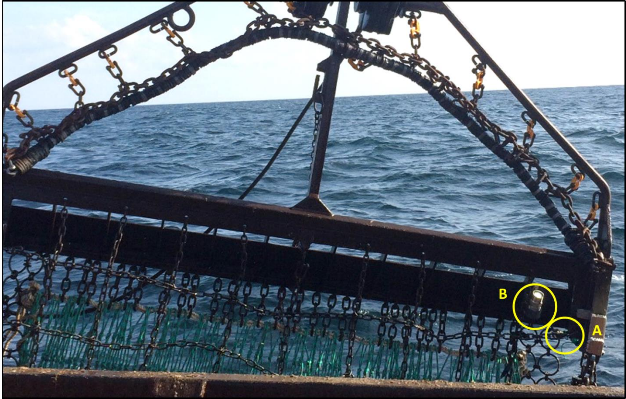
Figure 10. Image highlighting placement of GoPro HD action camera (A) and dive light (B) on F/V Let It Ride used to document FCS behavior in situ and fish interactions with the FCS. Camera and dive light were set up similarly on F/V Mister G .
