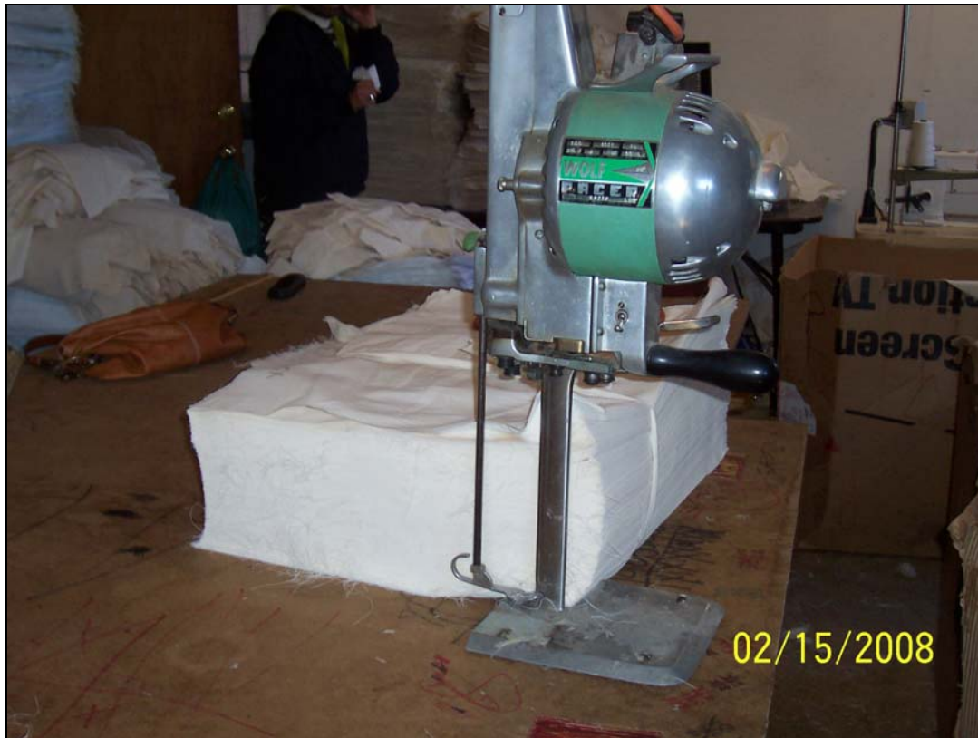
Fig. 7. Bolts of cloth are cut to the desired size.
