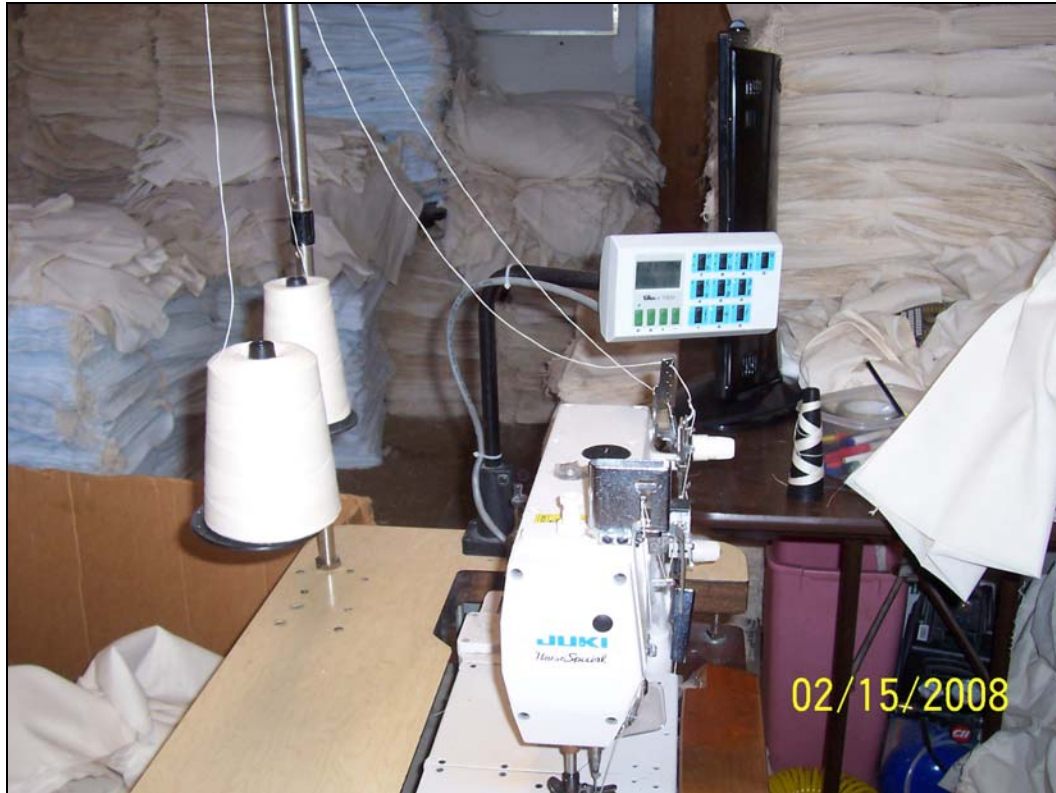
Fig. 9. The cloth is folded and the side and bottom stitched to form the bag by a computer assisted sewing machine.
