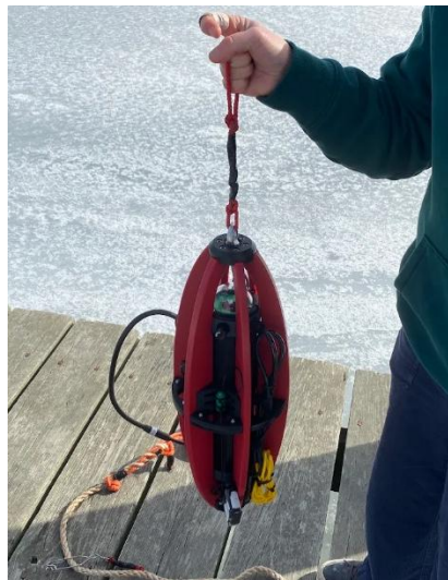
Figure 4. CFF's Remote Transmitter Sonde deployed during a test deployment to evaluate field performance prior to its routine use in future seasonal surveys.
