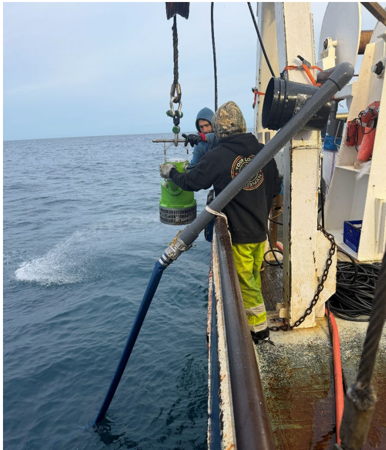
Figure 2. Two crew of the F/V Susan L prepare the Apex submersible pump to be deployed.
