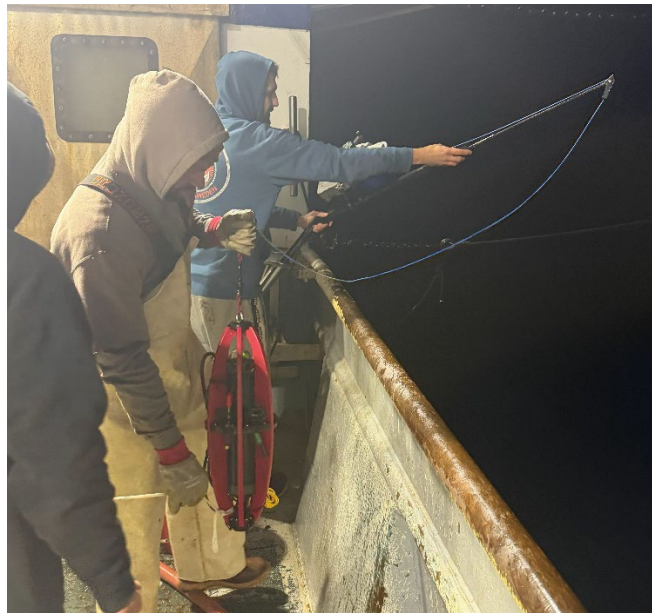
Figure 3. Crew of the FV Susan L preparing to deploy the Acbotics Research Fisherman's Sonde using an electric deepwater fishing reel and rod.
